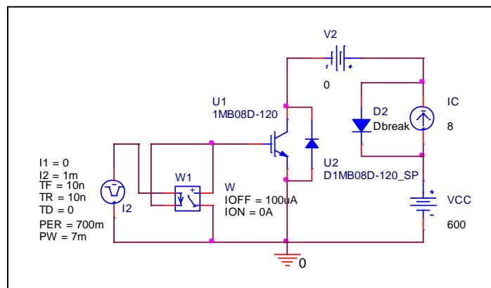
Test condition:  $V_{CC}=600$  (V),  $I_C=8$  (A),  $V_{GE}=15$  (V)
