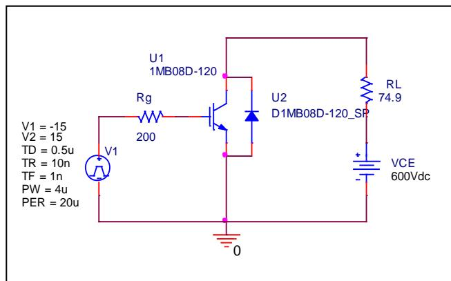
Test condition:  $I_C=8$  (A),  $V_{CC}=600$  (V)
