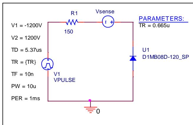
Test condition:  $Vcc=1200$  (V),  $Ic=8$  (A),  $-di/dt= 24$  (A/us)
